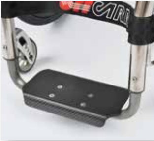
Pedana regolabile in inclinazione (optional) Tilt adjustable foot-plate (optional)
