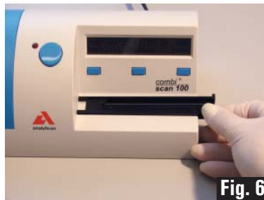
Fig. 6 Correct handling of the strip holder for positioning it into the device after cleaning.
